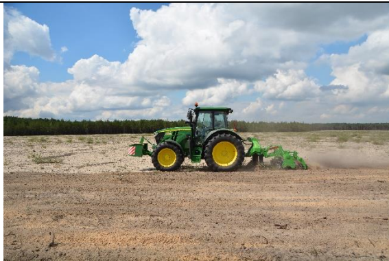
Works in the area with the use of subsoiler with tooth packer rollers (on the left), and sandcleaner (on the right) (Photo credit. Edyta Mazur)
