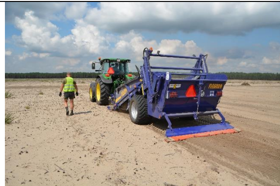
Works in the area with the use of subsoiler with tooth packer rollers (on the left), and sandcleaner (on the right) (Photo credit. Edyta Mazur)
